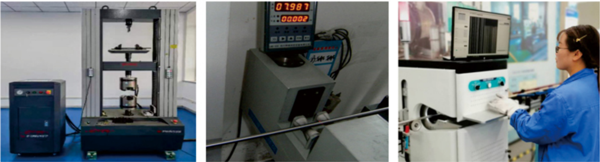
■ Microcomputer control electronic universal testing machine ■ Infra-ray diameter gauge ■ ODE optical surface detector
