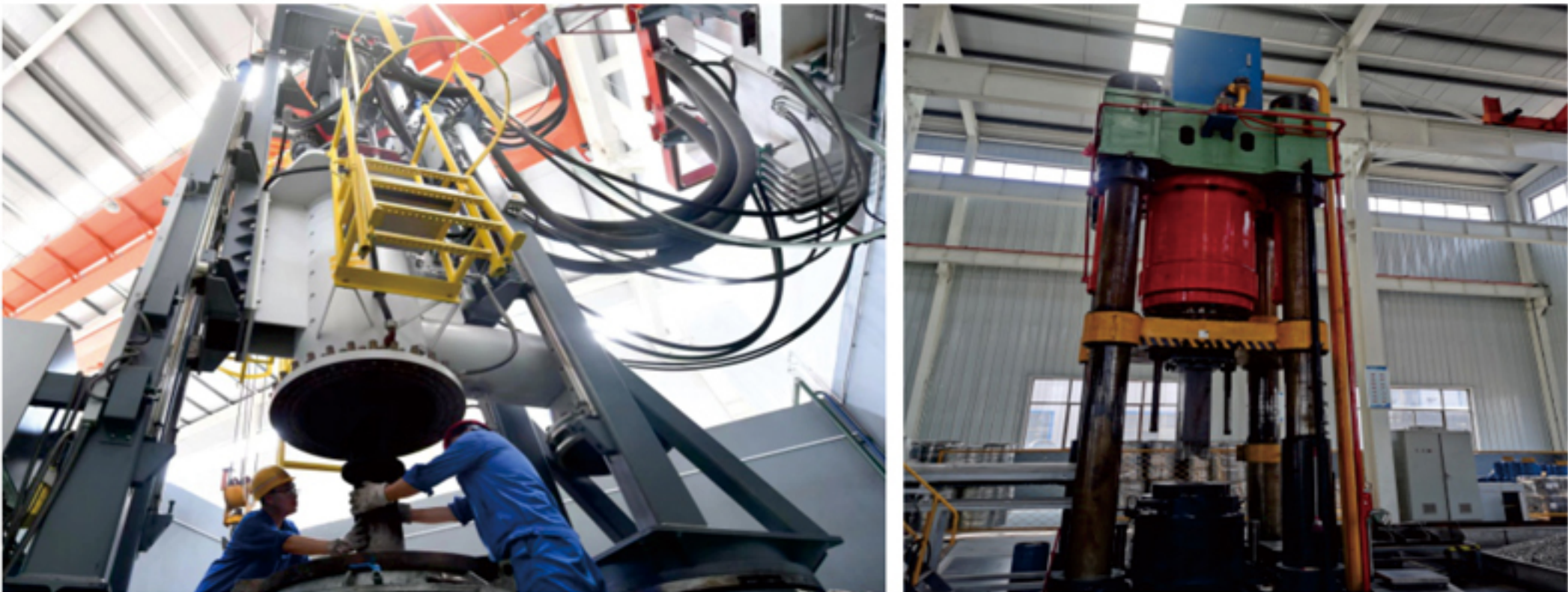
■ ALD vacuum melting furnace imported from Germany ■ 4500T hydraulic machine
